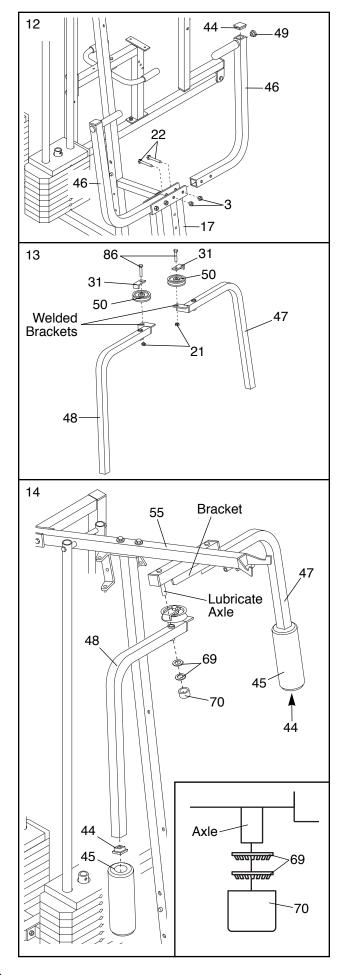
See the inset drawing. Attach the Military Press Arm (84) to the Pivot Arm (80) with two 5/16" x 2 1/4" Bolts (33) and two 5/16" Nylon Locknuts (3).
